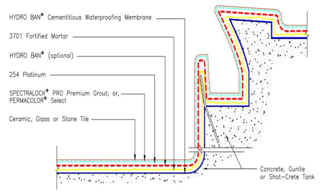
NOTE: Slurry Bond Coat of 254 Platinum is required under the mortar bed at all horizontal surfaces.
